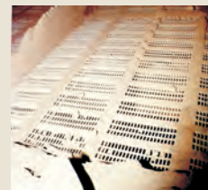
TIP TOP REMASCREEN stays almost completely clean thanks to its high selfcleaning effect.
