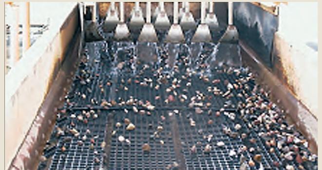
Longitudinally tensioned screen mat for the wet-screening of gravel.
