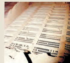
Steel screen mat shows 100% caking.
