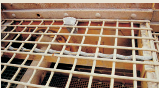
Wear to longitudinal bracings with a steel screen mat.
