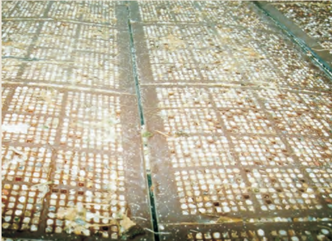
A traditional modular system showing almost 100% pegging.
